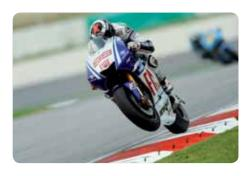
The front tyres will have a much easier time in Valencia than they did in Malaysia as, although twistier, the circuit is slower. Consequently the front slicks are available in softer specifications; the soft and medium compounds. The rear
