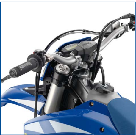
HANDLEBARS (FE, FS) A new handlebar is produced by Neken with the same bend as the predecessor which guarantees highest strength and safety.
